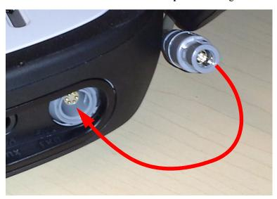
ECG Cable Connection to uSmart3300
