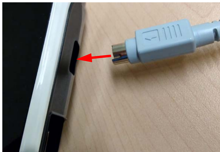
ECG Cable Connection to uSmart3200T
