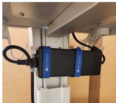
Mounting power supply on GCX cart
