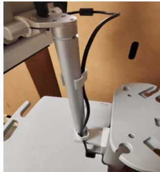
Mounting power supply on GCX cart
