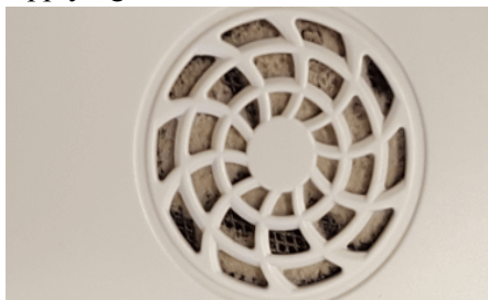
Clogged Cooling Vent
